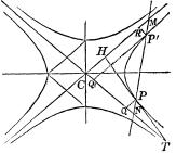
But x - x'' is equal to the sub-tangent QT: hence, the sub-tangent referred to the asymptotes, is equal to the abscissa of the point of tangency.
